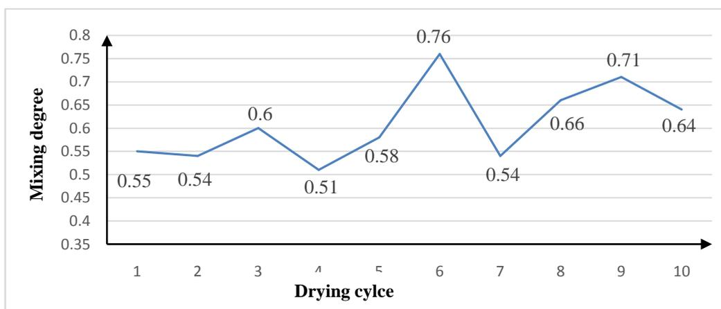
Fig. 4: Variation of the mixing degree for ten drying cycles with manual stirring
