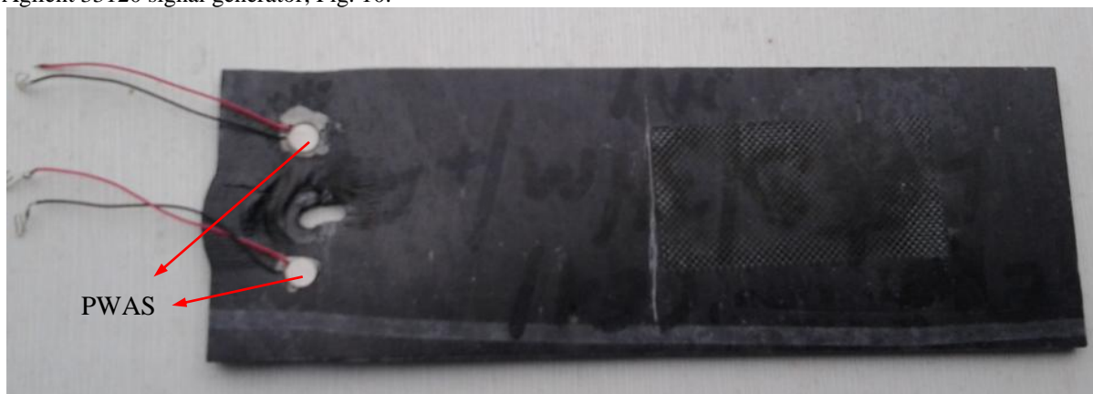
Fig. 9. PWAS positions on composite plate, geometry case 3
