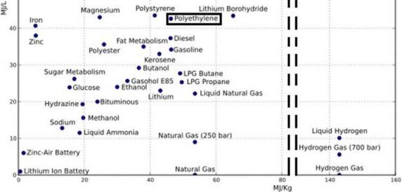
Figure 4: The energy densities of different materials (exception of oxidizing chemical agents) [20]
