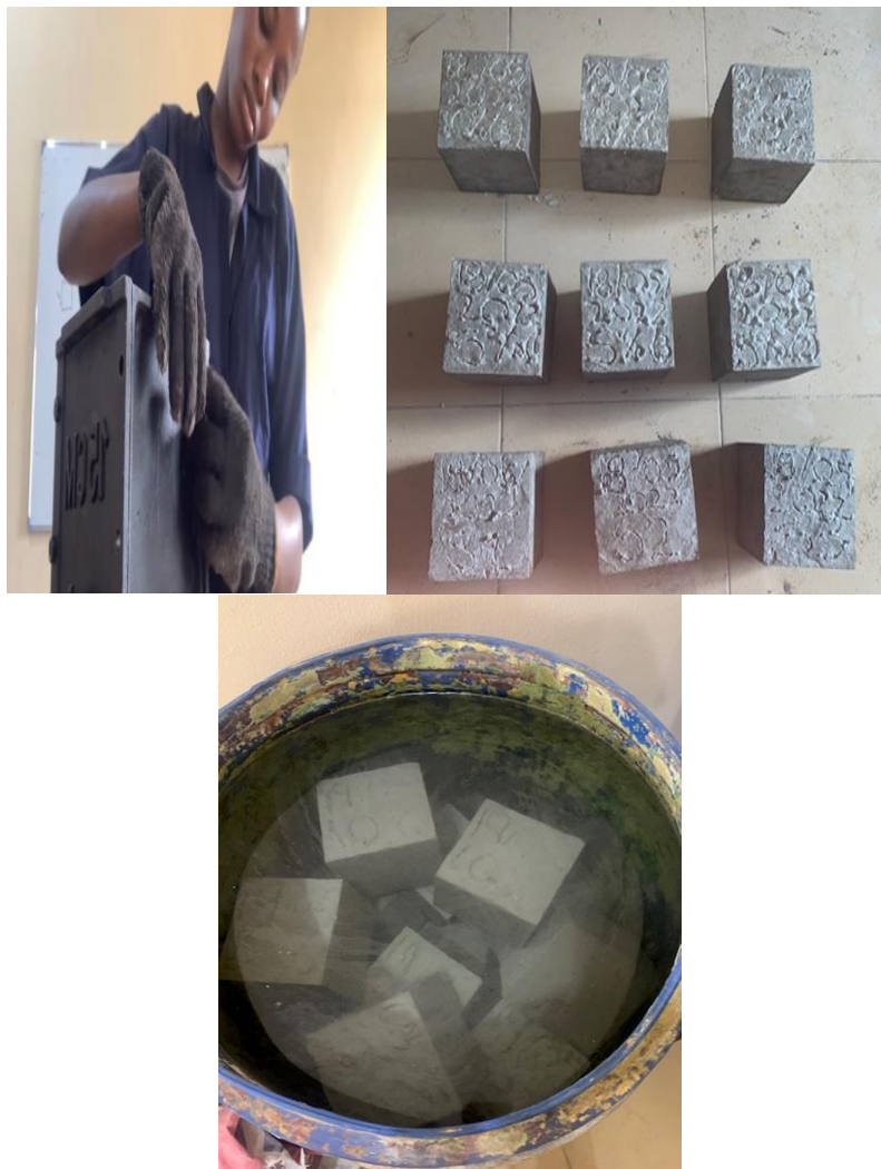
Figure 2: Demolding, sampling and curing of concrete cubes
