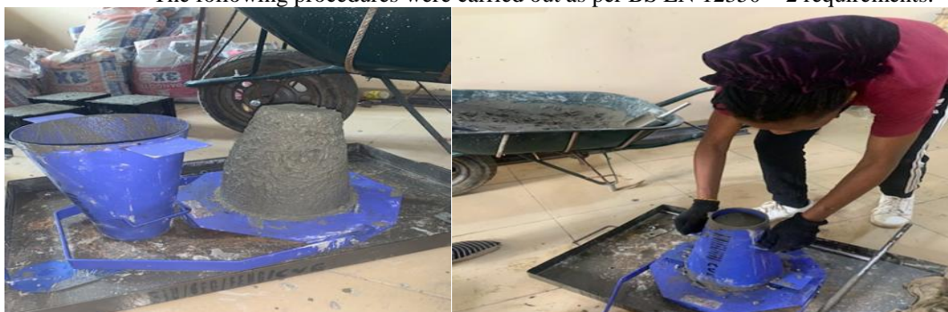
Figure 1: Conduction of slump test
