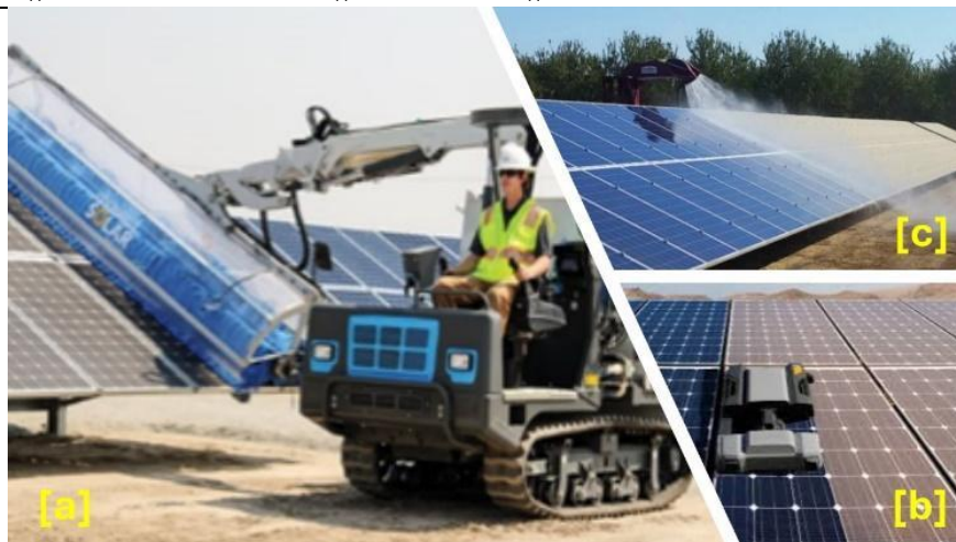
Fig. 2: a) MEGAWASH by Coldwell Solar b) EcovasRaybot c) Lectro Blaster Solar Cleaner
