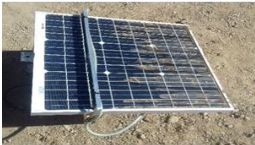
Fig. 8: Automatic solar panel cleaning system in operation
