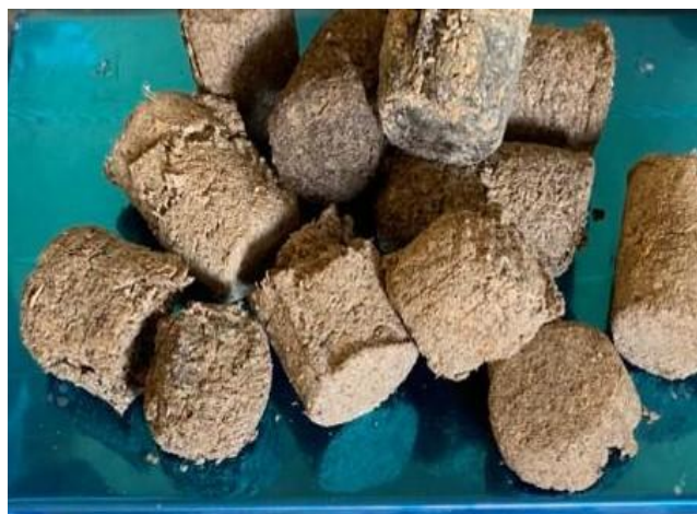
Figure 3: Briquettes produced from biomass
