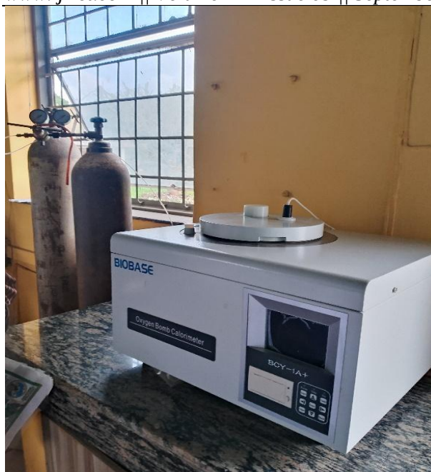
Figure 1: Bomb calorimeter testing equipment
