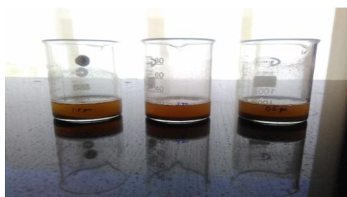
LSS solution used in order to exploit oil from the oil treated clay sample. The solution is opaque and muddy.
