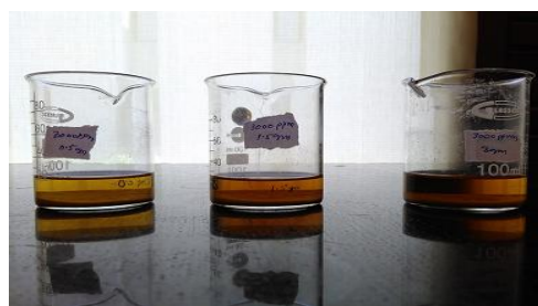
3000 ppm surfactant solution after leaving it for exploiting oil overnight
