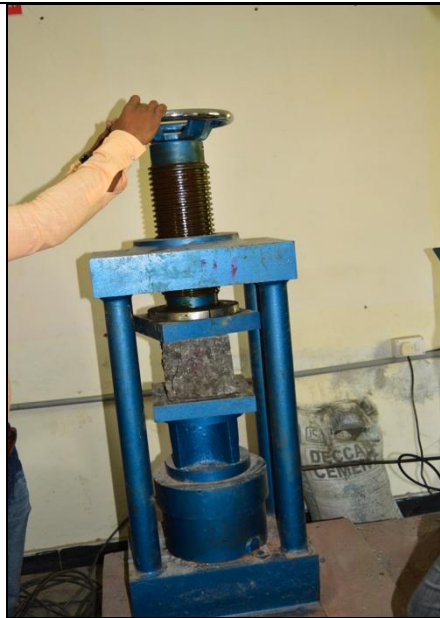
Fig 4.4: Compressive Strength Test Set Up for Cubes
