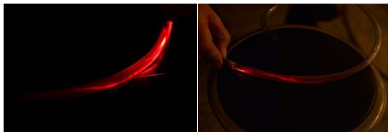
Figura 2. The illustration features a total internal reflection of the laser beam. Made in "FOTO SRETENOVIC". Photographer Vladimir Sretenović
