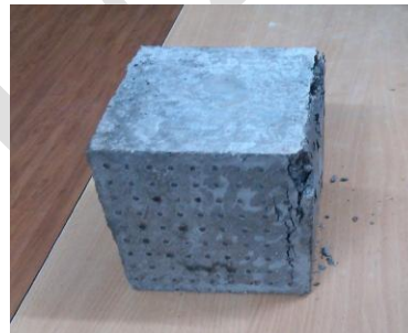
Fig. No. 4 Failure of Light Transmitting Concrete Cube
