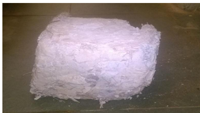
Fig. 8 Block after tested for compression
