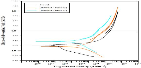
Fig 3: Cyclic polarization for the uncoated and (NiAl + YSZ) coated with different mixing ratios carbon steel in crude oil; Sweep rate 1 mV/sec.
