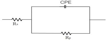
Fig4: Equivalent circuit to calculate the polarization resistance from impedance spectrum with a CPE: Rs - solution resistance between the reference electrode and the working electrode; CPE - the double layer capacity in parallel with the polarization resistance  $R_p$ .
