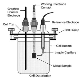
Fig(2): Schematic representation of a similar corrosion cell used for testing[13].
