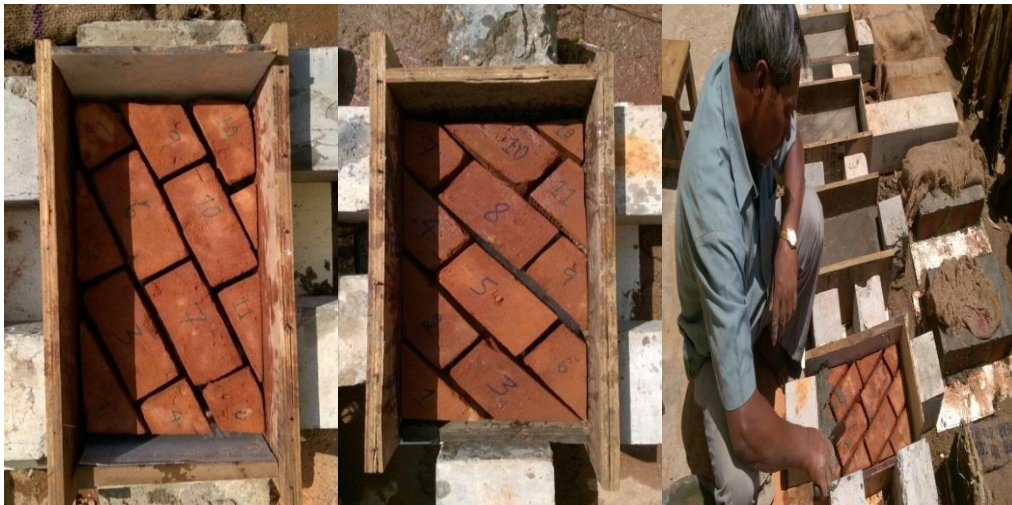
Fig 6 View of Cut TMBs Placed in Position Before Casting.
