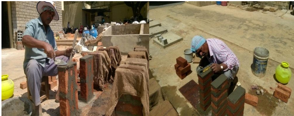
Fig 9 Prisms For Loading Parallel To Bed Joint.
