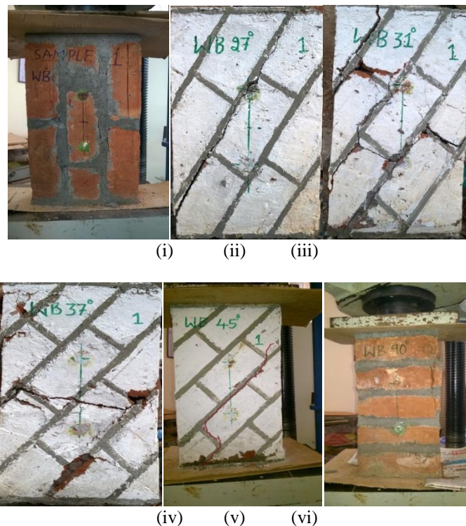
Fig 16: Failure Patterns of Wire Cut Brick Prisms Tested For Loading Conditions
