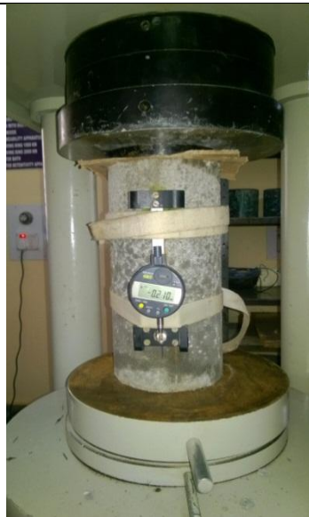
Fig 11 Mortar Cylinder Testing For MOE.
